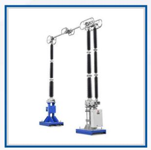
GÜRAL Knee-Type Disconnectors (HBD) help site designers to reduce area usage by the low projection area between the phases and let them have a choice to decide on two-layer busbar applications due to its reduced open-height in comparison with vertical-breaks thanks to the hinged main circuit arm.
